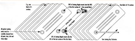
Please note that it is not advisable to exceed 20 (1200mm) sections in terms of assembly and handling. Assembly between 10 (600mm) and 35 (2100mm) sections is possible, however, please contact Sensotherm for additional advice.
