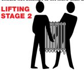
Always carry radiators vertically, never in a horizontal position - failure to carry correctly may cause water leaks.
